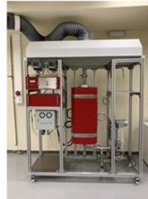
Micro-pilot unit fluidized bed/continuous pyrolysis reactor
