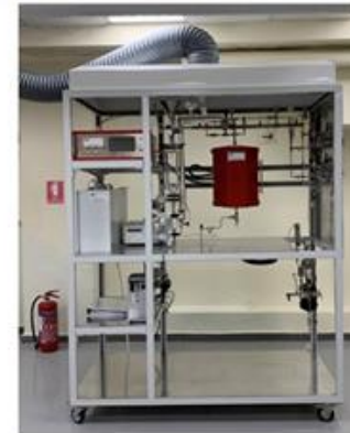
High-pressure, fixed-bed, continuous flow catalytic reactor (micro-pilot unit)
